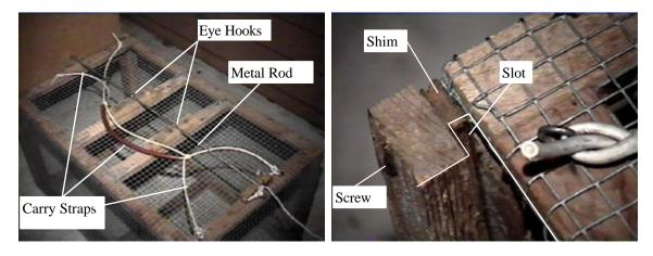
The photo on the left is a little closer view of the top of the trap, showing the metal rod, eye-screws, carrying strap, and hardware cloth. On the right you see a close-up of the slot fabrication located on the upper left-hand side of the door opening. The slot is outlined with white lines for clarity.
